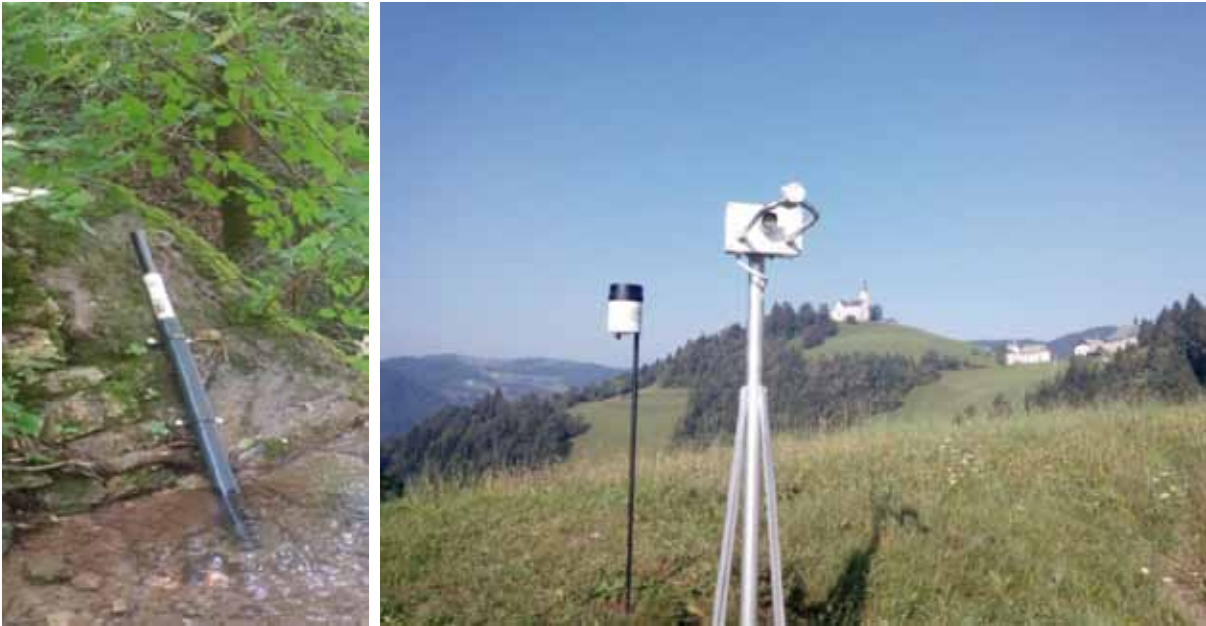
Figure - 4. The measuring equipment at the Gradaščica River experimental catchment (left: the suspended sediment probe; right: the disdrometer and a tipping bucket rain gauge).
