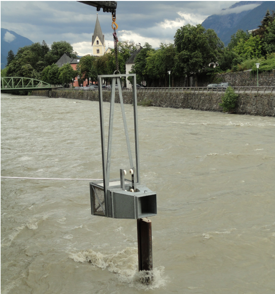
Figure 5: Bedload transport measurement with the TIWAG basket sampler at the Isel River in Lienz, Austria photo: Johann Aigner 2013 (BOKU University of applied sciences, Austria)
